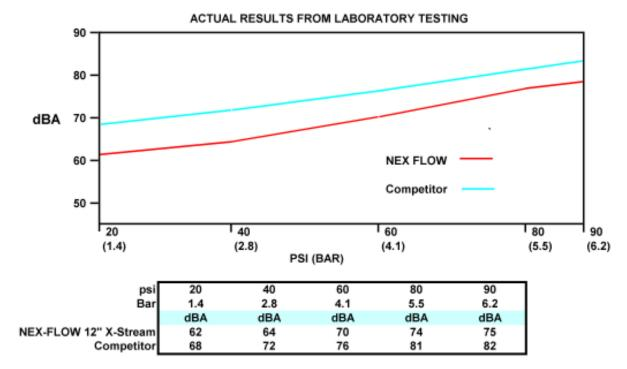
All Laboratory tests were conducted strictly in direct comparision with the same style of 12" (305mm) Air Knife from Competitor
